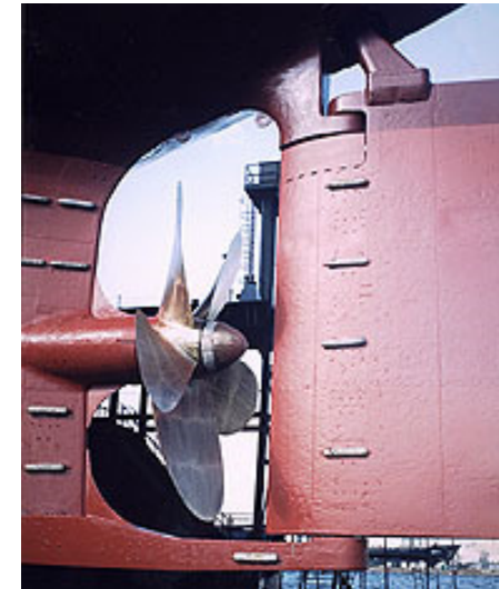
Cathodic protection with Zn sacrificial anodes
